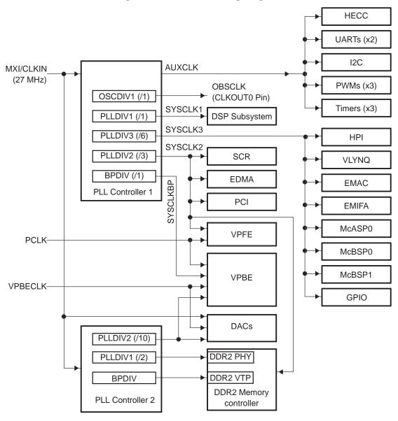
Figure 4-1. Overall Clocking Diagram
